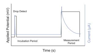
• *Incubation period:* After Drop Detect, glucose dehydrogenase catalyzes a selective electron-transfer reaction between glucose in the sample and  $M_{ox}$  (potassium ferricyanide) in the reagent layer:
