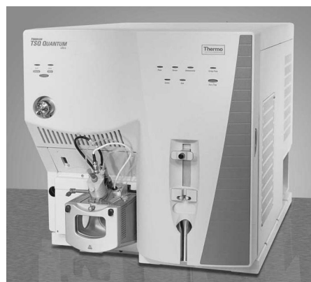
F11. The LC/MSMS TSQ Quantum Ultra equipped with ESI, APCI and APPI interfaces.
