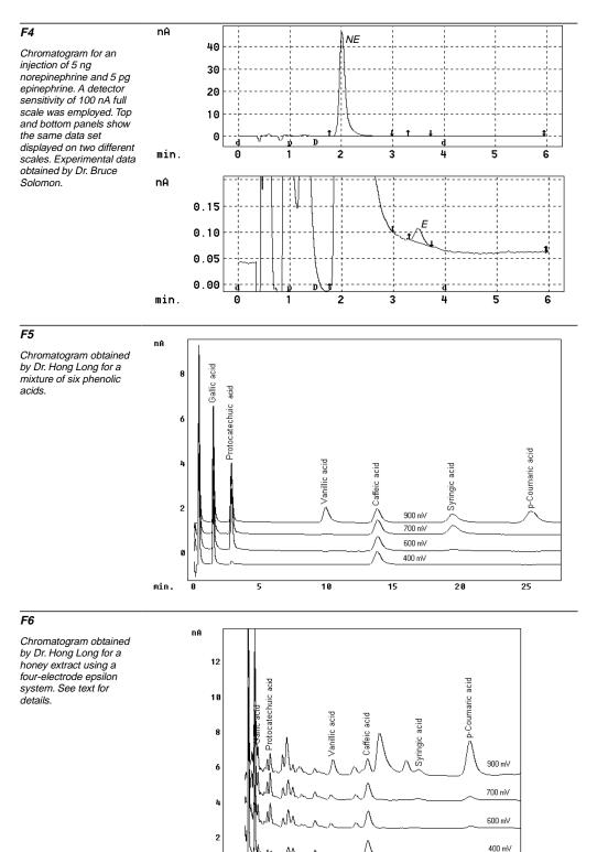
glassy carbon working electrodes in the arc configuration (see **F3**). For the first injection, the detectors were set to 300, 350, 400, and 450 mV (vs. Ag/AgCl). The detectors were reset to 500, 550, 600, and 650 mV for the second injection, and 700, 750, 800,
