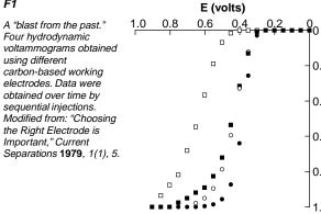
potential should be set to a value well positive of the observed half-wave potential of the analyte of interest to obtain maximum sensitivity (current per unit change in concentration).
