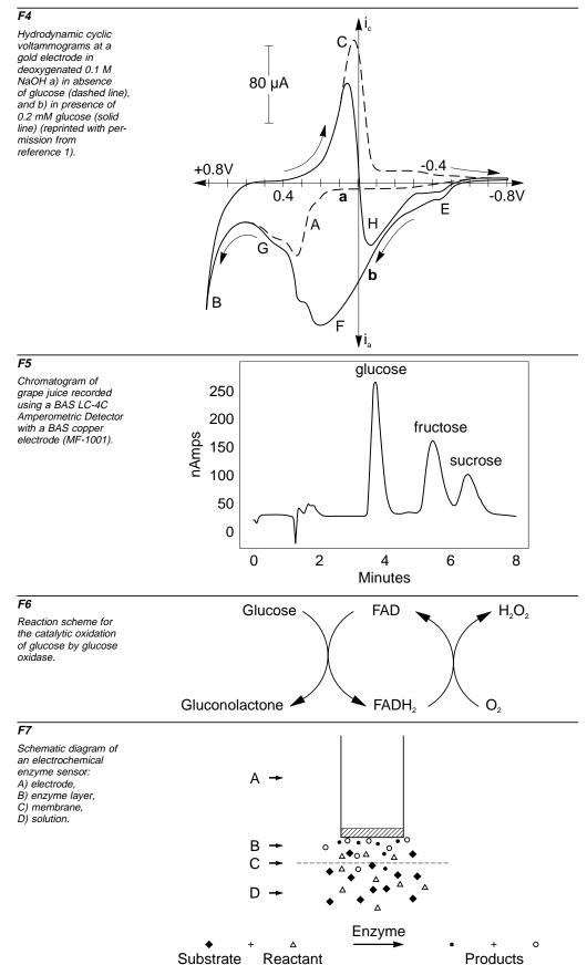
the surface of an electrode, and this immobilized layer is covered by a membrane. The function of the membrane is to provide stability, and it can also be used to prevent potential interferants from reacting with the enzyme. The electrode assembly is placed in the solution containing the analyte, which can readily diffuse through the membrane, and into the immobilized enzyme layer.
