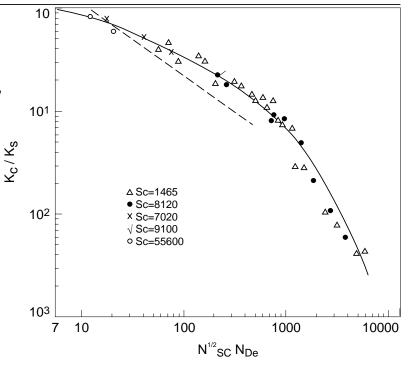
ing the reduction in dispersion associated with coiled tubes to the dimensionless  $DnSc^{1/2}$  parameter. However, no work has been done in the range of flow rates applicable to microbore chromatography. The following experimental evaluation attempts to rectify this problem by testing band spreading in open-tubular, helically coiled, and knitted reactors and comparing the results to the aforementioned solution.
