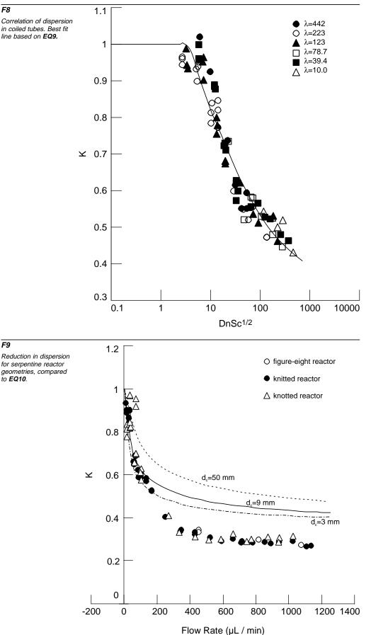
0.225 mm were coiled with a diameter of 2.25 mm, and the flow rate was 0.100 mL/min, the coiled-tube band spreading would be 56% compared to the straight tube case as calculated from **EQ10**. Therefore, the residence time for the reactor in this case could be 44% larger than in a similar straight tube yielding the same amount of band spreading.
